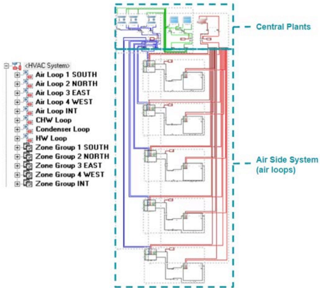
Figure 6: Schematic of variable air volume (VAV) system as modelled
