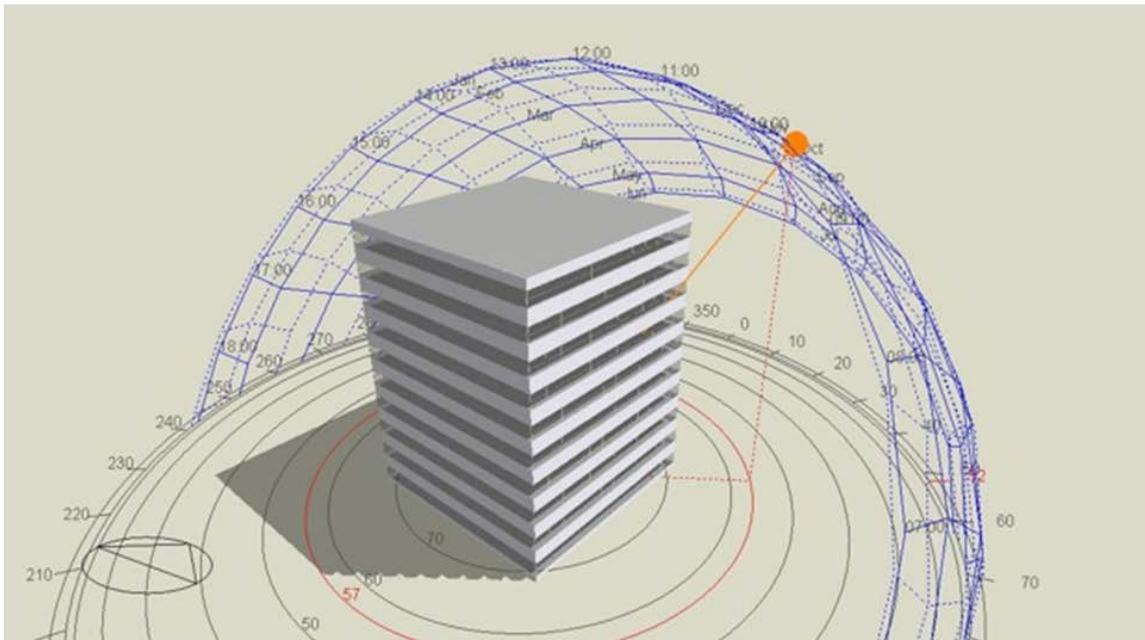
Figure 1: 3D visulation of the building with superimposition of annual sunpath for Sydney
