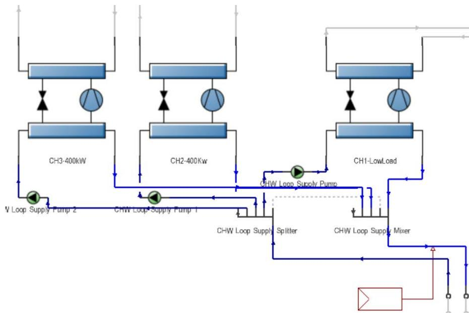
Figure 3: HVAC plant – chilled water (CHW) loop
