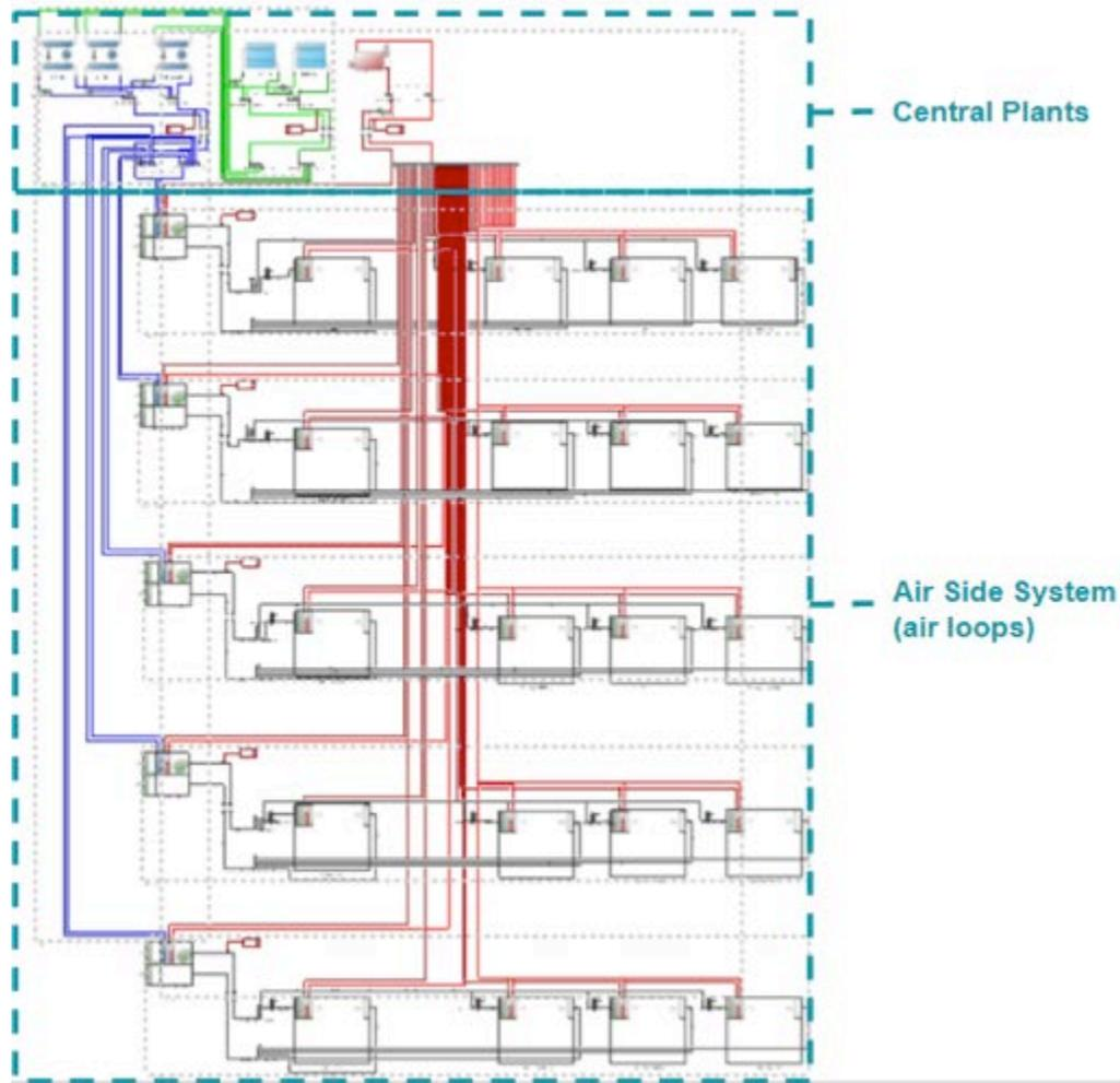
Figure 8: Schematic of Under Floor Air Distribution system as modelled
