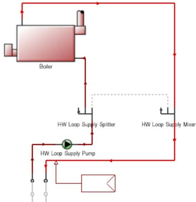
Figure 5: HVAC plant – heating hot water (HHW) loop
