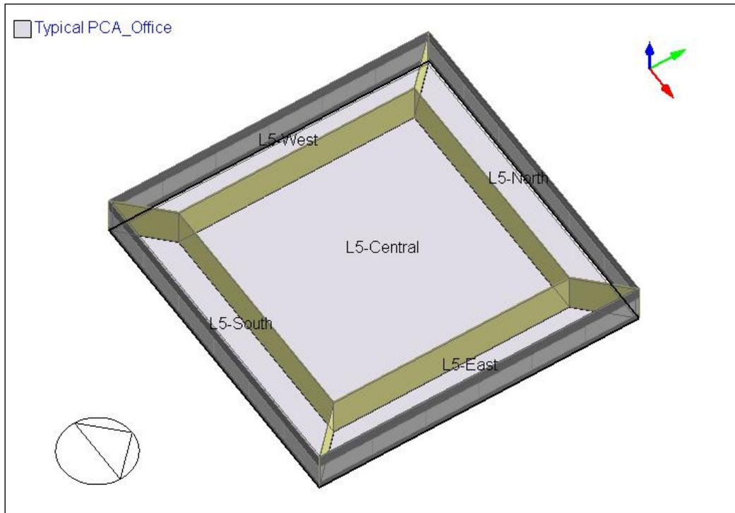
Figure 2: Zoning for typical floors; the zones are separated by “virtual walls”, ie., heat transfer boundaries, typically used in HVAC design for open plan offices
