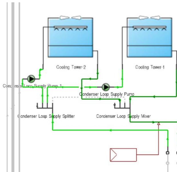
Figure 4: HVAC plant – heat rejection or condenser water (CW) loop
