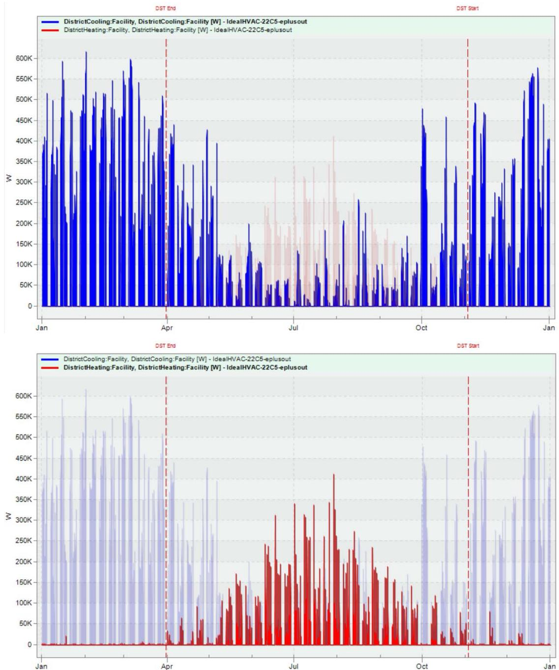
Figure 9a and b: Predicted building annual thermal cooling (above) and heating (below) hourly loads to be met by the HVAC systems being modelled, generated for a 22.5C setpoint. These loads are generated for the assumed operational profiles and are lower than the design day peak loads
